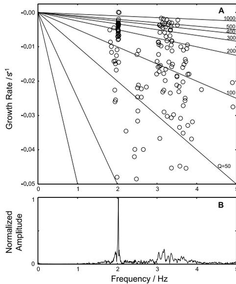
**Figure 3.** (A) Plots of the complex frequencies of individual wave elements for all the trial AR orders (4–60) estimated for the LP event that occurred at 7:48 (GMT) on 8 December 2001 shown in Figure 2. (B) Amplitude spectrum estimated for this event.
