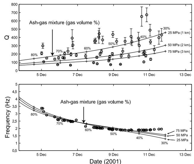
**Figure 4.** Temporal variations in frequency and  $Q$  determined for LP events. The solid lines show the best fits of frequency and  $Q$  calculated for a crack containing the ash-gas mixture at various pressures between 25 and 75 MPa corresponding to the source depths between 1 and 3 km below the summit, in which we assumed the crack lengths of 200, 230, and 240 m at the depths of 1, 2, and 3 km, respectively.
