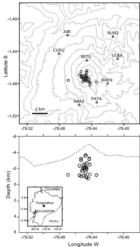
**Figure 1.** Hypocenters (open circles) of the LP events and location of seismic stations (open triangles) operated by the Instituto Geofísico, Escuela Politécnica Nacional. The inset shows the location of Tungurahua Volcano in Ecuador.
